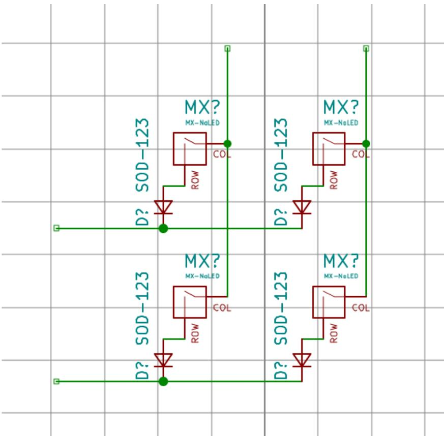
Finally, add global labels for each row and column. It is recommended to label them counting from 0 up, since that is how it is handled firmware side as well.
