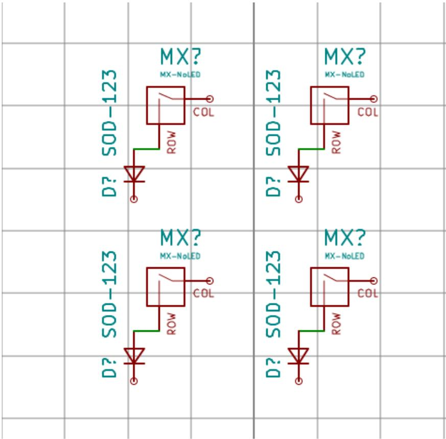
Then, drag a wire across the diode cathode and COL pins of each row and column, and terminate them using the hotkey k:
