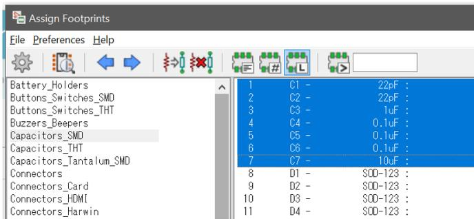
Then double click the 0805 footprint in the right panel to assign the C\_0805\_2012Metric footprint to all capacitors.
